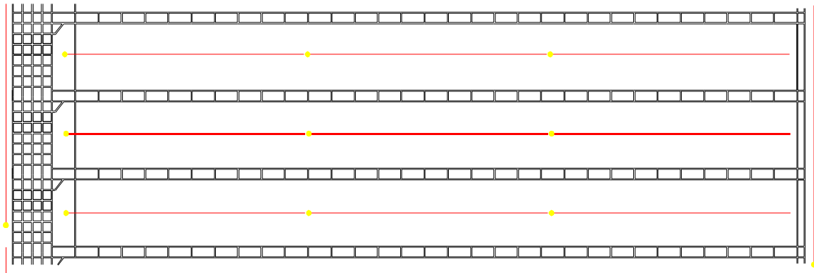
Figure 7 Example MRD Pattern, High Permeability and/or Long Lead Time
